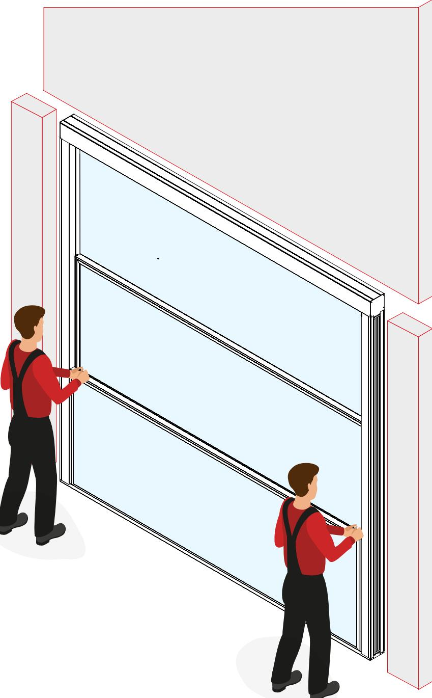
Reassemble the **AL11** and **AL13** covers, which we separated from the box profile in the first stage. At first **AL11** and then **AL13** are mounted as shown in the picture.
